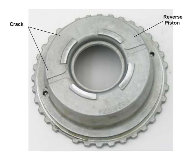
The updated Reverse Piston is thicker and can be identified by a larger chamfer.
