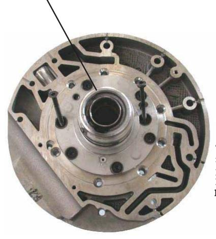
This alignment dowel is used to align the pump halves. VERY IMPORTANT not to lose it. **IMPORT**
