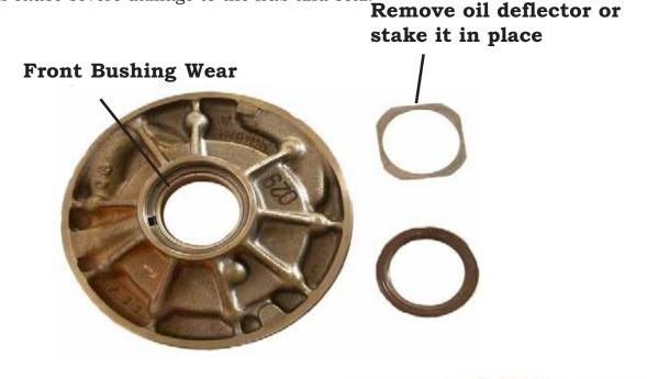
Possible front seal leak due to the oil deflector becoming loose and damaging the seal
