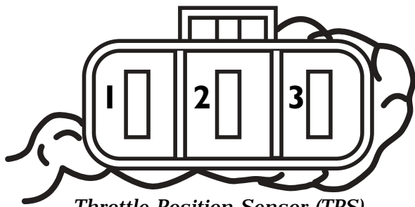
Throttle Position Sensor (TPS) harness connector shown from the switch side of the connector
