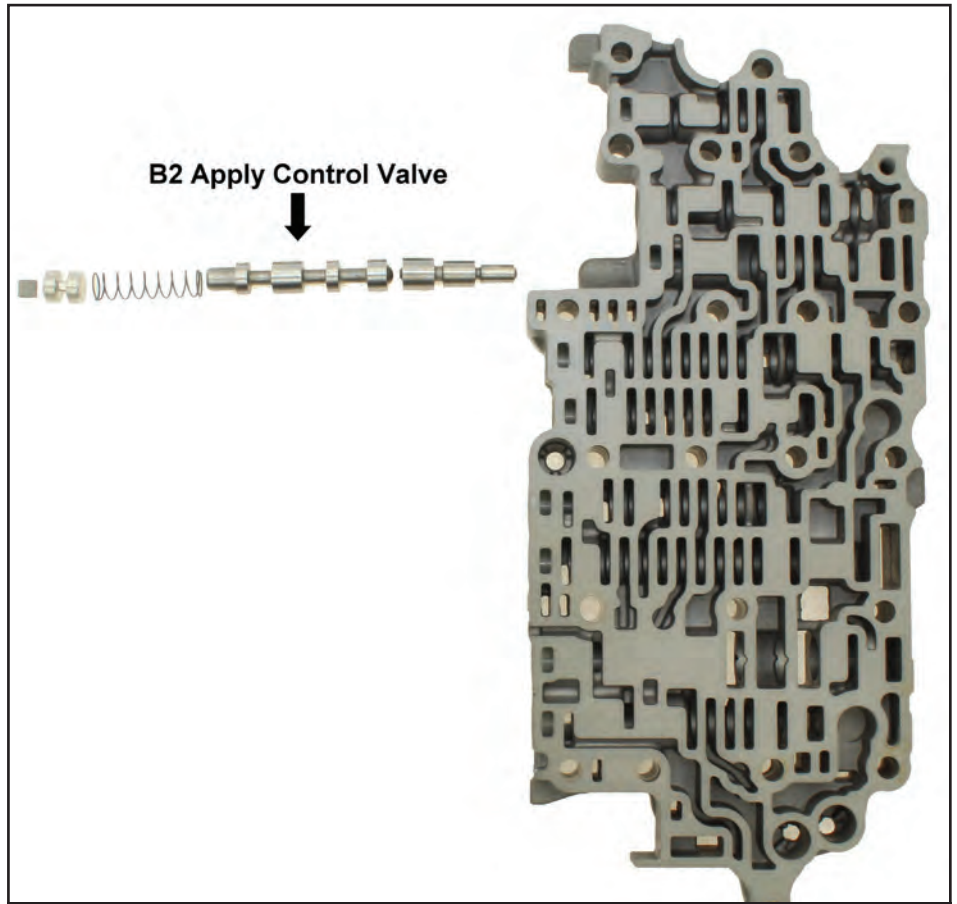
Figure 2: Worn B2 Apply Control Valve
